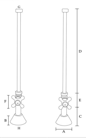
(A) Flange: 2-1/2" OD (D) Tube: 24" L (G) Connection to the faucet: 1/2"; 14 threads/in.
