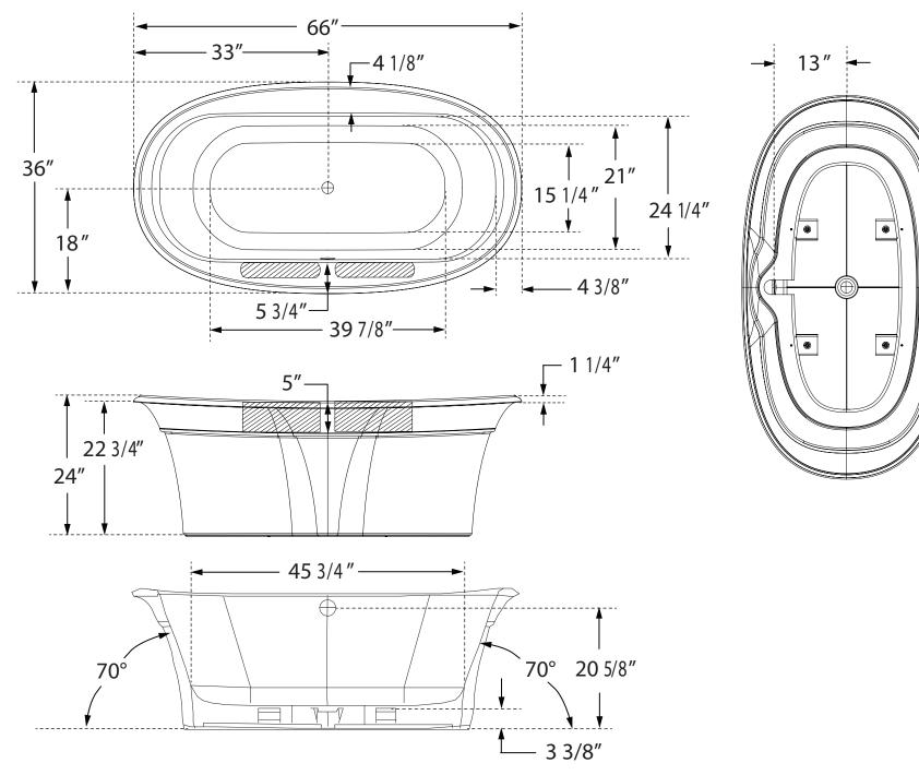
: Recommended faucet area 2 sections of 10" (L) x 2 1/2" (W) Depth recommended for straight pipes 5".
