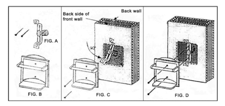
Installation clamp with spring (Fig. A) for easy installation of recessed bathroom accessories (Fig. B).
