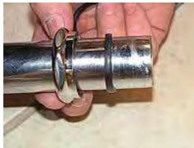
11. The "T" is then screwed to the connecting pipe with the longer side of the "T" in the upward direction in order to give you enough room to adjust the overflow tube/receiver.
