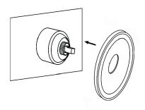
3. Remove the decorative screw cover from the valve randle. Slide the handle orto the valve stem and secure it by tightening the set screw with the provided hex wrerch. Reinsert the screw cover to conceal the screw. 4. Slide the decorative back plate onto the shower arm, and install the shower arm by threading it into its prepared female fitting. Apply thread sealant or plumber's tape to the threads before tightening. Install Hand tighten firmly.
