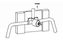
IMPORTANT: COMPLETE THE CONSTRUCTION OF YOUR WALL, INCLUDING ANY FINISHED WALL MATERIALS SUCH AS TILE. BEFORE PROCEEDING WITH THE REMAINDER OF THE INSTALLATION.
