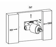
3. Route, assemble, and connect all in-wall piping to and from the shower valve Make connections appropriately depending upon the type of pipe that is being used For copper pipe, soldering will be required and should be completed by a licensed plumber. Apply plumber's tape to any threaded connections if applicable. Install any wood blocking that is necessary to support the piping and valve.
