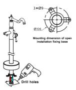
7. Install expansion screws fix the faucet component.
