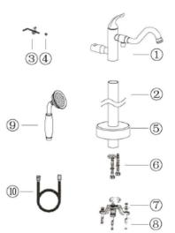
Step 1: Connect the hot and cold water supply lines (6) to the faucet body (1) and tighten. Slip straight riser tube (2) into floor escutcheon(5)
