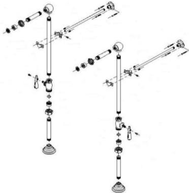
1. Note the rough-in centers for these supply lines are determined by the centers of the faucet they are being installed on. This faucet unit has 3 3/8" centers.
