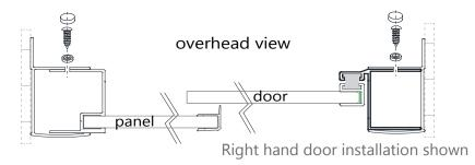
**21.** Apply a good quality mildew-resitant silicone around the interior perimeter along both walls and the threshold. **(Fig 21)**
