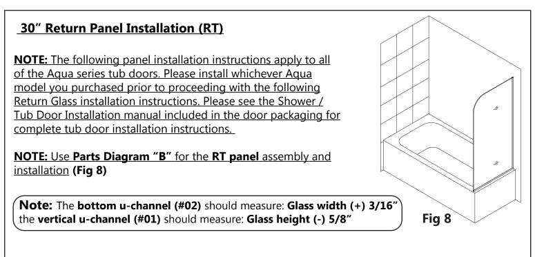
7. Slip the U-Channel 2 (bottom profile) (#02) and U-Channel 1 (wall profile) (#01) onto the Return Panel Glass (#03).
