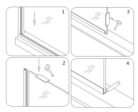
Adjust the **Support bar** to a proper position on the **Stationary glass (03)** and the wall. Level it horizontally. Hold it firmly and outline the bracket's position on the wall. Remove the **Support bar** and detach the wall bracket from it. Place the bracket against its outlined position on the wall and mark the drilling hole.
