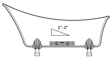
15. Place a level inside the tub. Make sure the bathtub is stable and that all legs rest perfectly on the floor, if not, ad-just the levelling pads.
