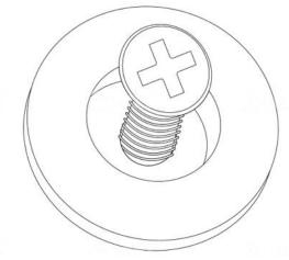
13. Secure the 4-floor leveler disc to the floor with the screws.
