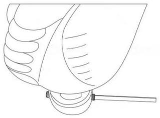
14. Place the bathtub in its position and tighten the set screws on the 4 leveling pads to the floor leveler disc using the allen key
