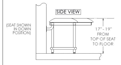
With the seat in the down position, level the seat by changing the adjustable rubber feet to the desired mounting height (17"-19"). Tighten the lock nuts.
