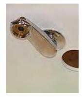
5. Apply the jam nut / lockdown nut to the back of the faucet nipple. (Do not tighten yet).
