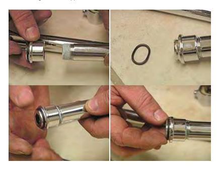
5. Place allen wrench into allen opening and strap wrench to tighten valve end to nipple until tightened.
