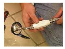
25. Attach small lock nut side of hose into cradle inlet. Hand tighten a 1/4 turn using the smooth jawed pipe wrench.
