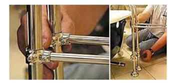
18. Hand-tighten valve lock nut then tighten 1/4 turn with smooth jawed wrench.
