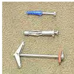
5. Place a toggle bolt to the back of the sink.
