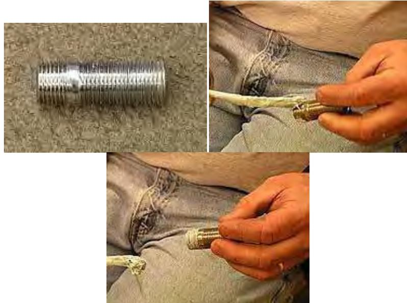
2. Tighten the faucet nipple to the 1/2" thread on the deck mount coupler. You want to hand tighten a 1/4 turn using the strap wrench.
