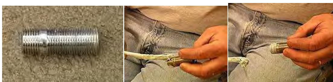
5. Tighten the faucet nipple to the 1/2" thread on the deck mount coupler. You want to hand tighten a 1/4 turn using the strap wrench.
